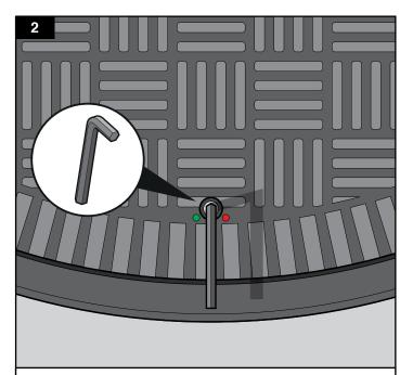
Insert the the Allen key so the top bar is between the green and red dots.
