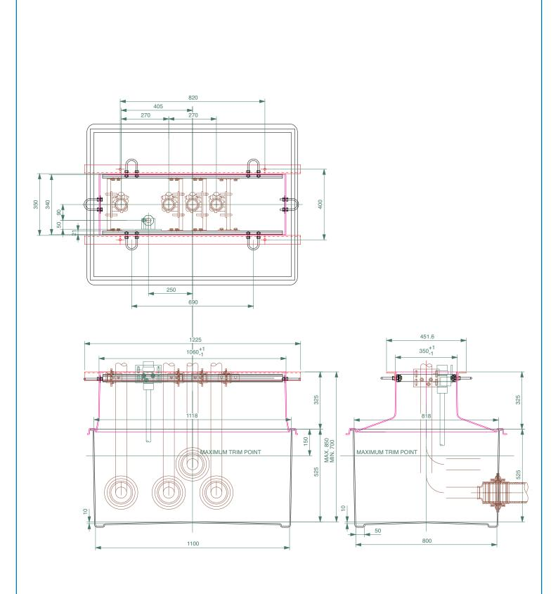
1100mm x 800mm GRP solid base sump and corbel to fit Censtar CS42 series models. Metalwork included.
