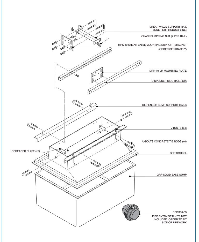
1100mm  $\times$  800mm GRP solid base sump and corbel to fit Censtar CS42 series models. Metalwork included.
