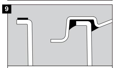
Apply a bead of sealant to the top of the sump flange. If this has been removed during trimming, apply sealant inside the groove of the corbel. Position the corbel onto the sump and push down firmly.
