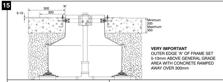
Concrete island depth fixed as per architect drawing. Allow concrete to cure
