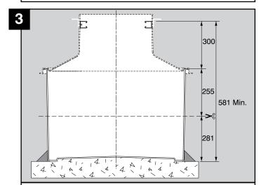
Sump can be trimmed to reduce the height of the system by up to 255mm, if 150mm holes will be drilled for pipe entry kits.
