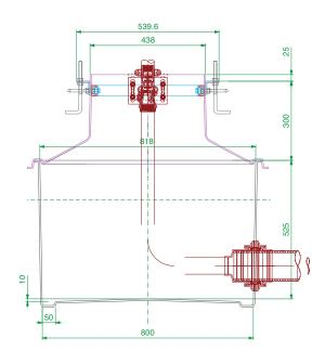
1100 x 800mm GRP solid base sump and corbel to fit Gillbarco dispenser model Encore 500. 4 Product. Includes dispenser support rails, shear valve rails and all fixings. Metalwork reference SIM322.
