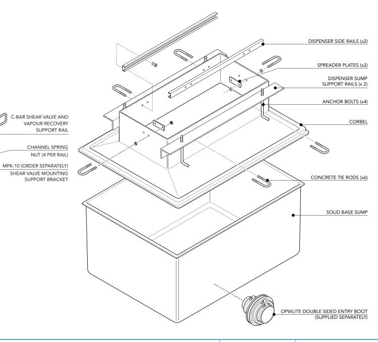
1100 x 800mm GRP solid base sump and corbel to fit Gillbarco dispenser model Encore 500. 4 Product. Includes dispenser support rails, shear valve rails and all fixings. Metalwork reference SIM322.
