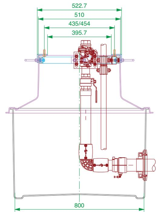
1100mm x 800mm GRP solid base sump and corbel to fit Gilbarco SK700 1/2 dispenser model. Includes dispenser support rails, shear valve rail and all fixings. KPS pipework and Fibrelite entry boots.
