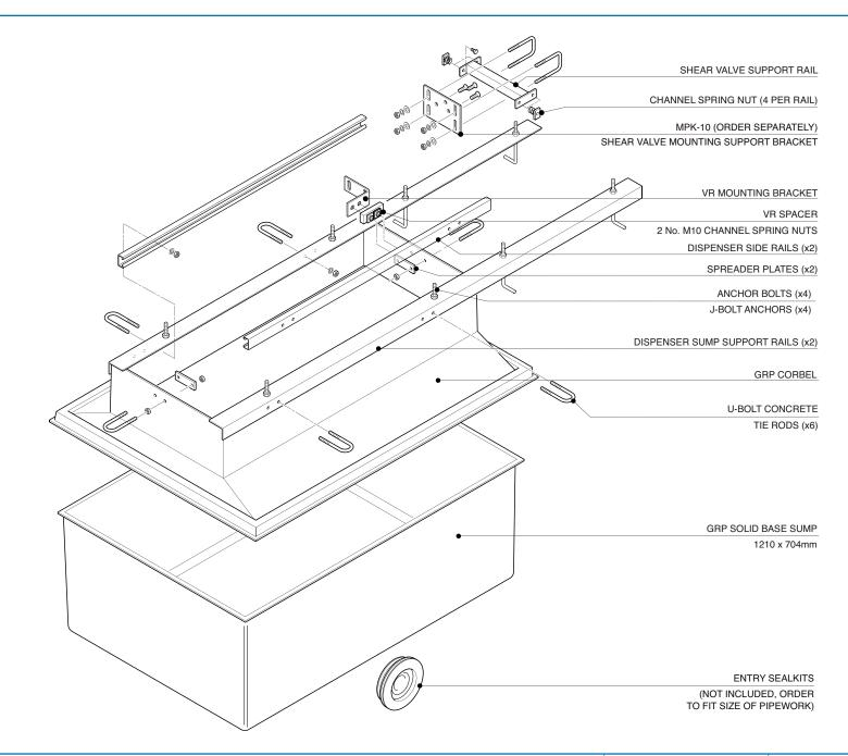
1210 x 704mm GRP solid base sump and corbel to fit Gilbarco SK700 II 4/8 dispenser model. Includes dispenser support rails, shear valve rail and all fixings. KPS pipework and Fibrelite entry boots.
