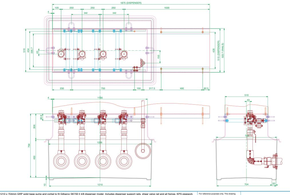
1210 x 704mm GRP solid base sump and corbel to fit Gilbarco SK700 II 4/8 dispenser model. Includes dispenser support rails, shear valve rail and all fixings. KPS pipework and Fibrelite entry boots.
