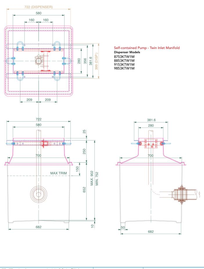
$682 \ x \ 682 \ x \ 652 \ m \ deep$  dispenser sump and corbel to fit Gasboy TW1 dispenser models. Includes dispenser support rails, 1 shear valve rail and all fixings.
