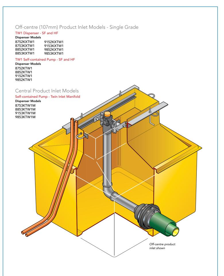
682 x 682 x 652mm deep dispenser sump and corbel to fit Gasboy TW1 dispenser<br/>models. Includes dispenser support rails, 1 shear valve rail and all fixings.F
