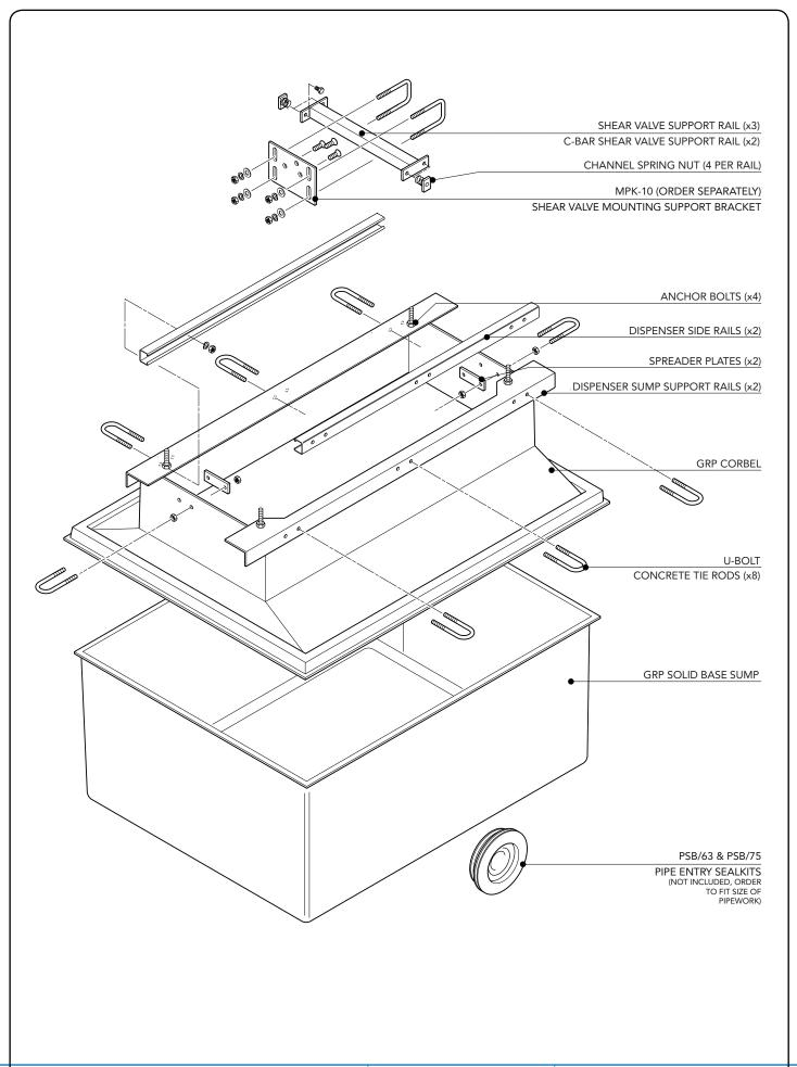
12 10mm x 704mm GRP solid base sump and corbel to fit Tokheim Quantium Q410 dispenser model. Includes dispenser support rails, 5 shear valve rails and all fixings. 8 Hose version.
