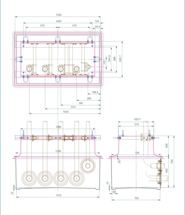
1210mm x 704mm GRP solid base sump and corbel to fit Tokheim Quantium Q410 dispenser model. Includes dispenser support rails, 5 shear valve rails and all fixings. 8 Hose version.
