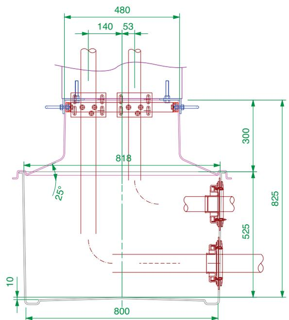
1100mm x 800mm GRP solid base sump and corbel to fit Tokheim Quantum Q510, 4-6. Includes dispenser support rails, 3 shear valve rails and all fixings.
