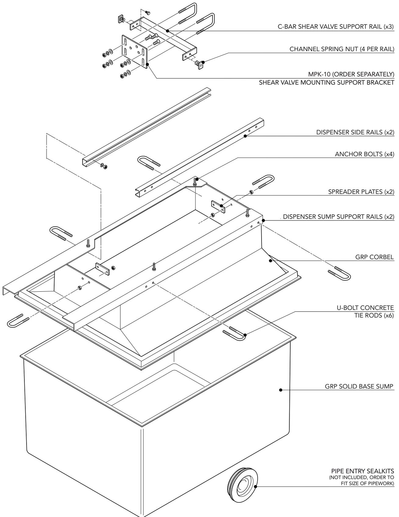
1100mm x 800mm GRP solid base sump and corbel to fit Tokheim Quantum Q510 , 4-6. Includes dispenser support rails, 3 shear valve rails and all fixings.
