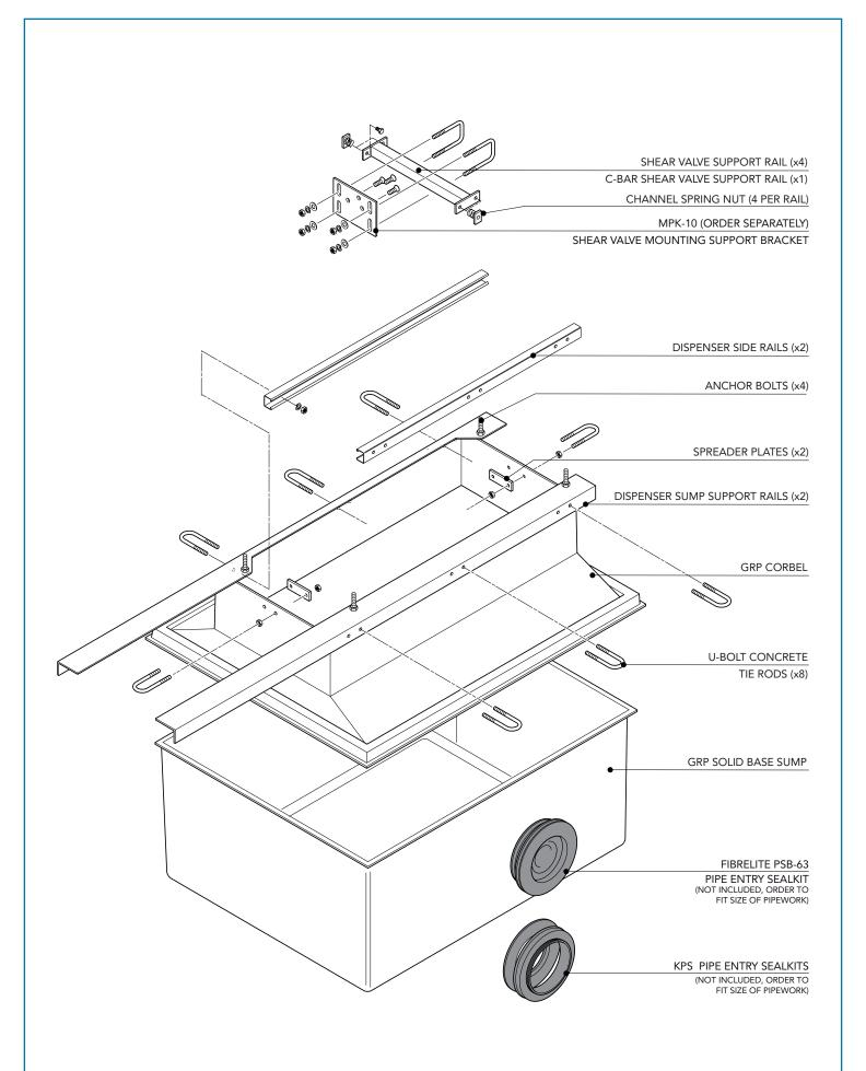
$\frac{1210\times704\text{mm}}{1200\times704\text{mm}}$  GRP solid base sump and corbel to fit Tokheim Quantium Q510 , 4-4, 4-8. Includes metal work.
