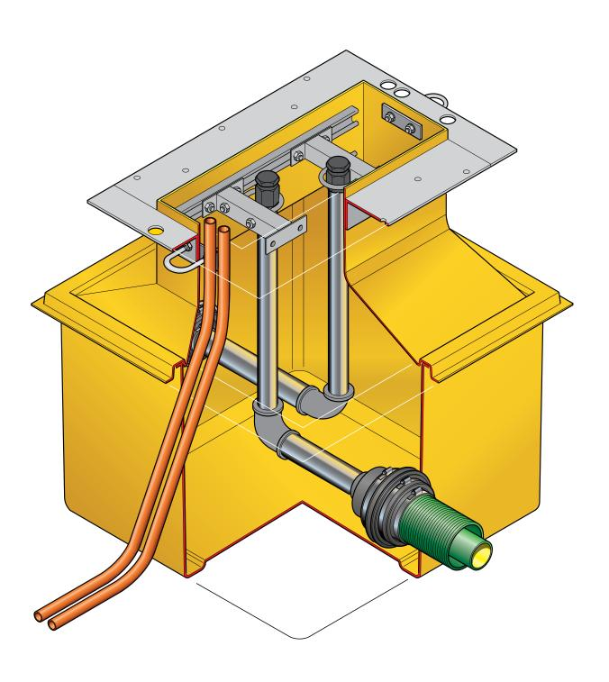
$682 mm \ x \ 682 mm \ GRP$  solid base sump and corbel to fit Tatsuno CR Sunny model 222/LPO (2 product). Includes dispenser support framework, 10 'J' bolts, 6 concrete tie rods and 2 shear valve rail.
