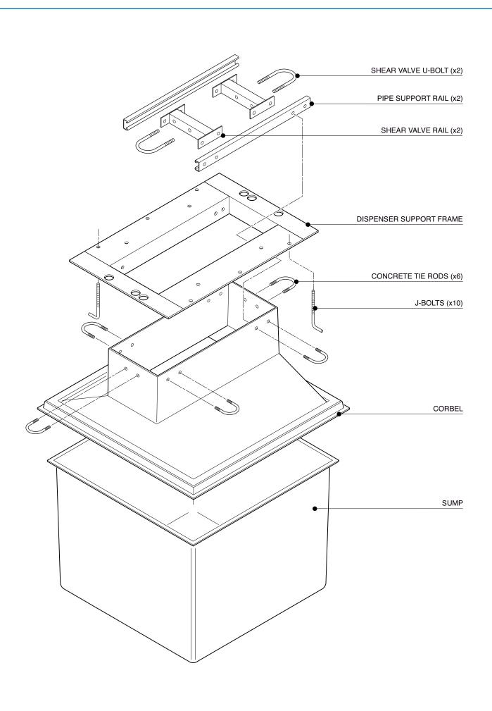
682mm x 682mm GRP solid base sump and corbel to fit Tatsuno CR Sunny model 222/LPO (2 product). Includes dispenser support framework, 10 'J' bolts, 6 concrete tie rods and 2 shear valve rail.
