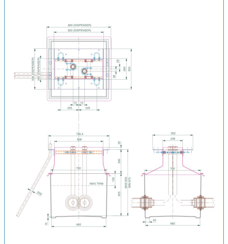
682mm x 682mm GRP solid base sump and corbel to fit Tatsuno CR Sunny model 222/LPO (2 product). Includes dispenser support framework, 10 'J' bolts, 6 concrete tie rods and 2 shear valve rail.
