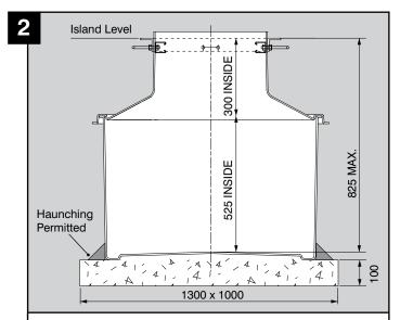
Dry fit the corbel on top of the sump to check level and prepare a adequate support base.
