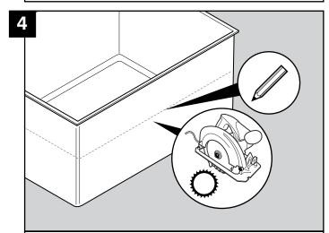
Mark trim point around the sump. Check position of pipe entry sealkits before trimming with a circular saw.
