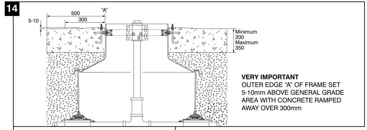
Concrete island depth fixed as per architect drawing. Allow concrete to cure
