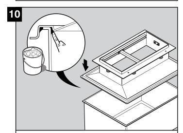
Apply sealant to BOTH the internal and external joint between the sump and corbel. Smooth off and press into the joint with soapy water to remove trapped air. Allow 12 hours for the sealant to set.
