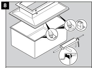
Abrade internal groove of corbel and top edge of the sump (inside & outside) with sandpaper. Degrease with acetone.
