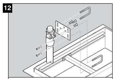
Complete pipework and secure to shear valve rails with the MPK-10 mounting kit. Refer to the shear valve arrangement plan detail on page 1.
