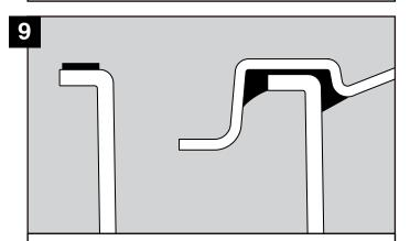
Apply a bead of sealant to the top of the sump flange. If this has been removed during trimming, apply sealant inside the groove of the corbel. Position the corbel onto the sump and push down firmly.
