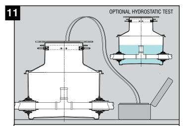
Optional vacuum water or hydrostatic test. Ensure pipework is capped off below the upward riser. Tighten clips on pipe entry sealkits against the pipe. Tighten nuts on upper support frame metalwork. Vacuum test at 0.6m depth setting only.
