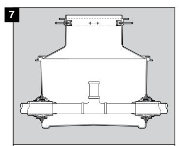
Run pipework through side wall, connect to upward riser. Cap off pipework to allow vacuum testing in Stage 8.
