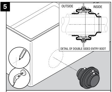
For PSB 50 to 110, PSBD 50 to 110 and PDBD pipe entry kit models a 150mm hole should be drilled. Mark up hole positions as illustrated.
