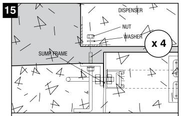
Remove upper nut & washer on the 4 anchor bolts Install & connect the dispenser to the sump frame & anchor bolt. Fit & tighten nut & washer.
