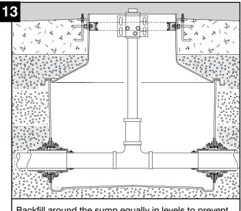
Backfill around the sump equally in levels to prevent uneven load against the sump wall.
