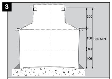
Sump can be trimmed to reduce the height of the system by up to 150mm, if 150mm holes will be drilled for pipe entry kits.
