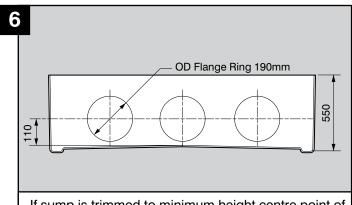
If sump is trimmed to minimum height centre point of hole is 110mm from base internally.
