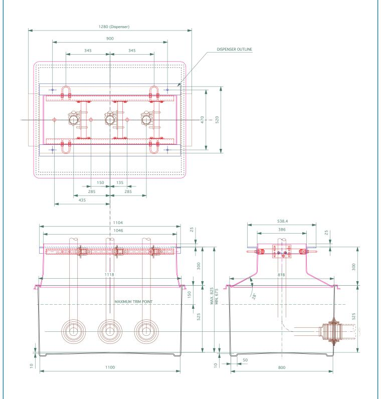
1100mm  $\mathbf x$  800mm GRP solid base sump and corbel to fit NEOSUNNY models. Includes metal work.
