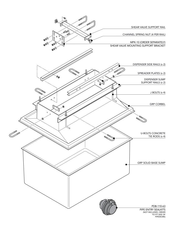
1100mm  ${\rm x}$  800mm GRP solid base sump and corbel to fit NEOSUNNY models. Includes metal work.
