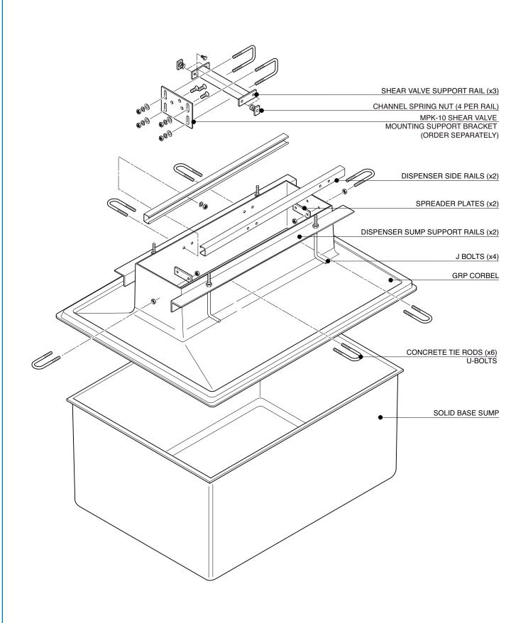
1100mm x 800mm GRP solid base sump and corbel to fit Tatsuno Salemaker 6 hose, 3 product models SM1060. Includes dispenser support framework, 6 'J' bolts, 6 concrete tie rods and 3 shear valve rails.
