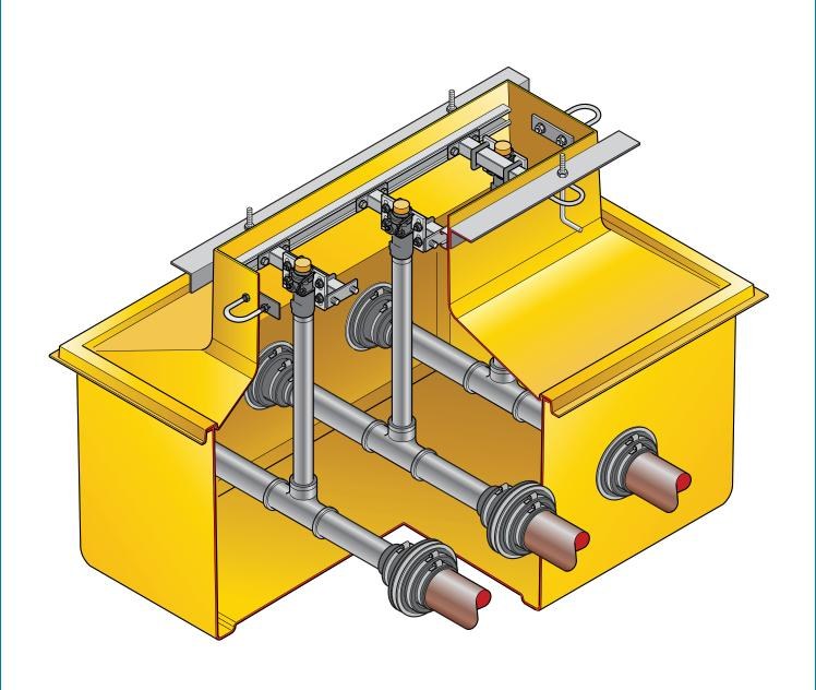
1100mm x 800mm GRP solid base sump and corbel to fit Tatsuno Salemaker 6 hose, 3 product models SM1060. Includes dispenser support framework, 6 'J' bolts, 6 concrete tie rods and 3 shear valve rails.
