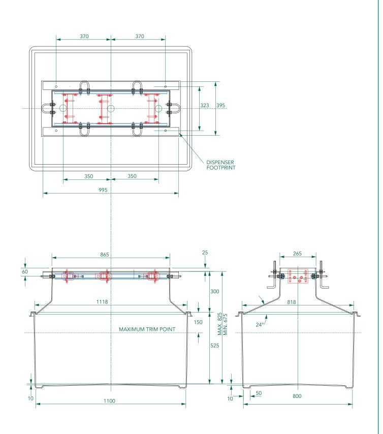
1100mm x 800mm GRP solid base sump and corbel to fit Tatsuno Salemaker 6 hose, 3 product models SM1060. Includes dispenser support framework, 6 'J' bolts, 6 concrete tie rods and 3 shear valve rails.
