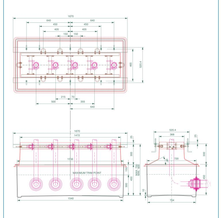
1556mm x 720mm FRP solid base sump and corbel with dispenser framework and 5 shear valve rails to fit Tatsuno Sunny XE model. Fits 5 product lines. Order MPK-10 shear valve rail mounting bracket separately.
