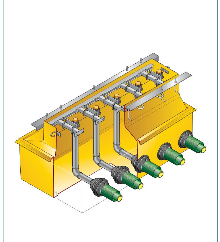
1556mm x 720mm FRP solid base sump and corbel with dispenser framework and 5 shear valve rails to fit Tatsuno Sunny XE model. Fits 5 product lines. Order MPK-10 shear valve rail mounting bracket separately.
