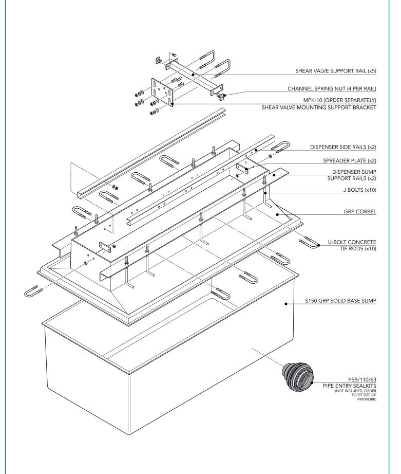
1556mm x 720mm FRP solid base sump and corbel with dispenser framework and 5 shear valve rails to fit Tatsuno Sunny XE model. Fits 5 product lines. Order MPK-10 shear valve rail mounting bracket separately.
