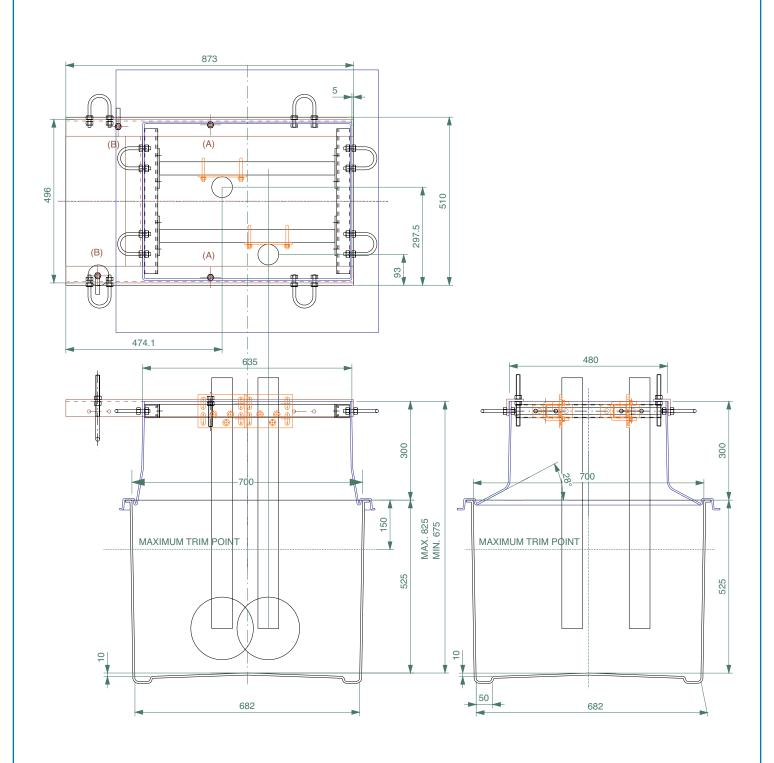
$682\text{mm}\ x\ 682\text{mm}\ \text{GRP}$  solid base sump and corbel to fit GobalStar 4 Hose dispenser.
