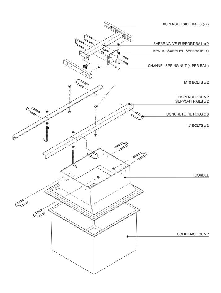
$682\text{mm}\ x\ 682\text{mm}\ GRP$  solid base sump and corbel to fit GobalStar 4 Hose dispenser.
