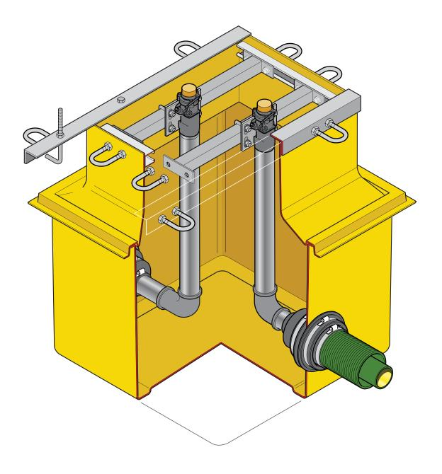
$682\text{mm}\ x\ 682\text{mm}\ \text{GRP}$  solid base sump and corbel to fit GobalStar 4 Hose dispenser.
