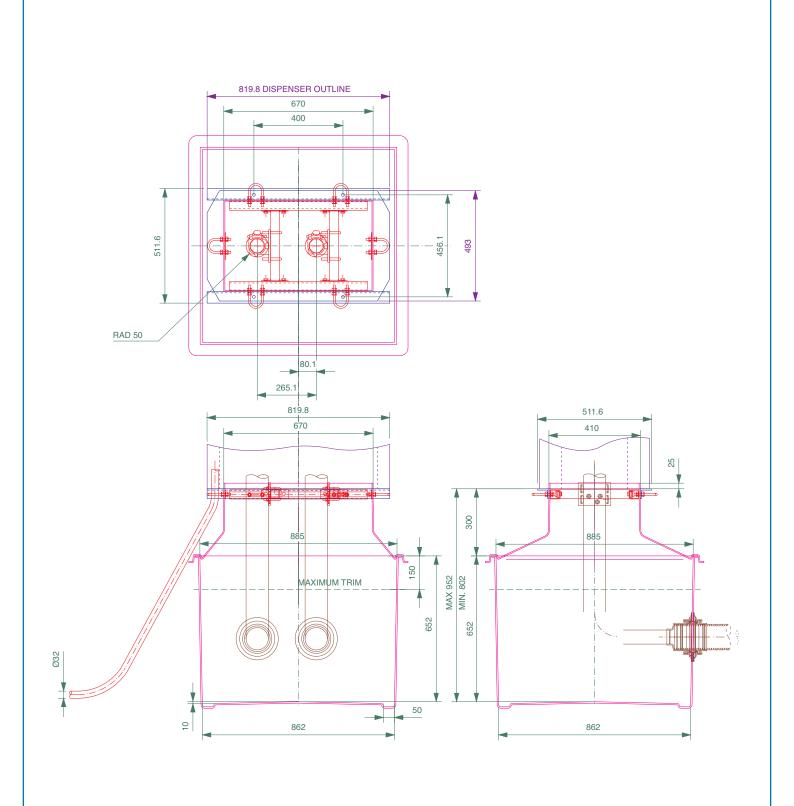
$862 mm \times 862 mm$  GRP solid base sump and corbel to fit Wayne Global Century 62200 model. Includes dispenser support rails, 2 shear valve rails and all fixings.
