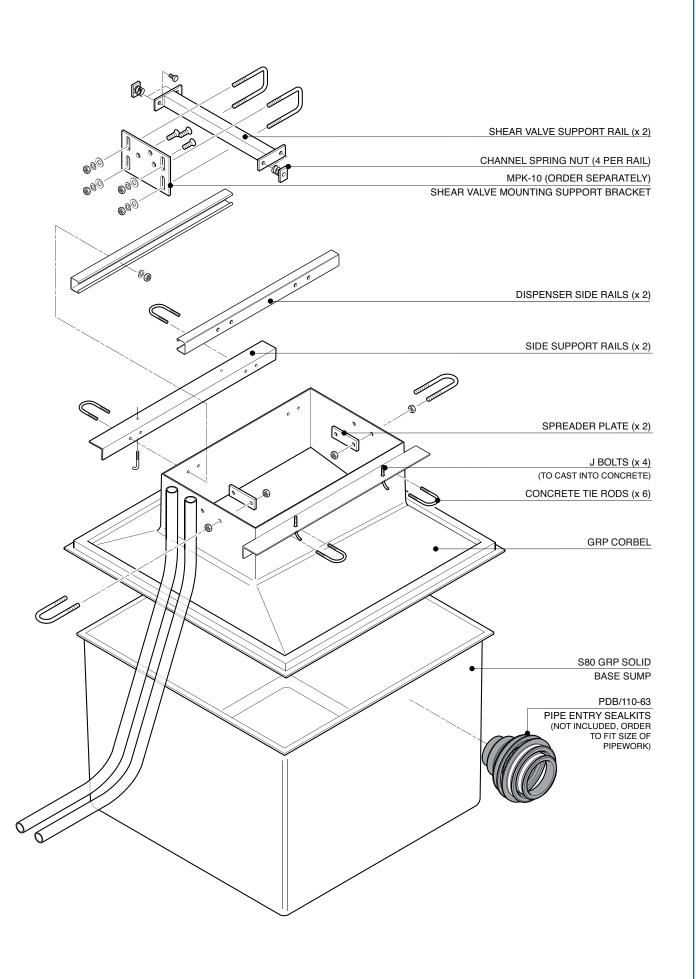
$862 mm \times 862 mm$  GRP solid base sump and corbel to fit Wayne Global Century 62200 model. Includes dispenser support rails, 2 shear valve rails and all fixings.
