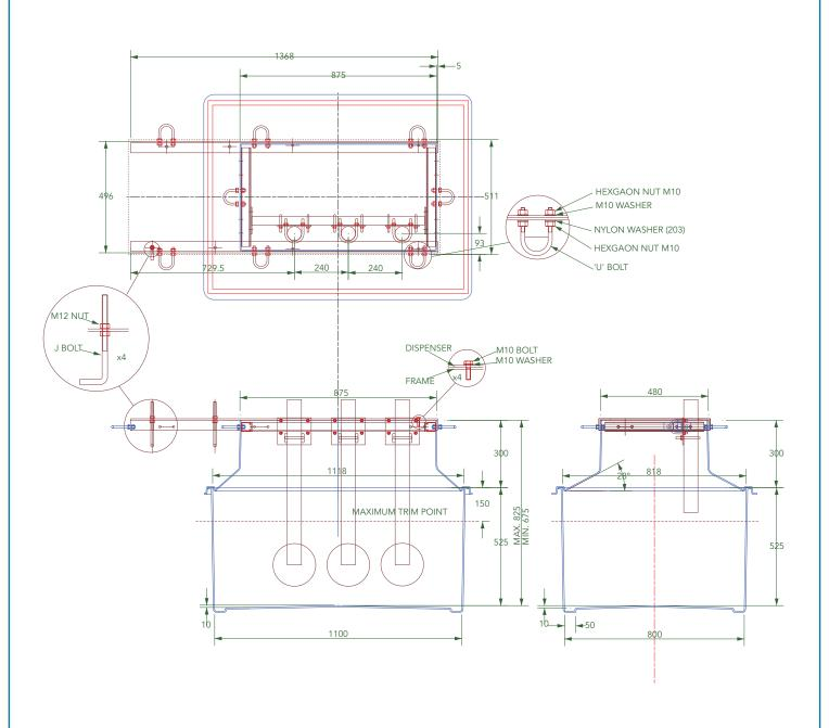
1100mm x 800mm GRP solid base sump and corbel to fit GobalStar 6 Hose dispenser. Side rail version.
