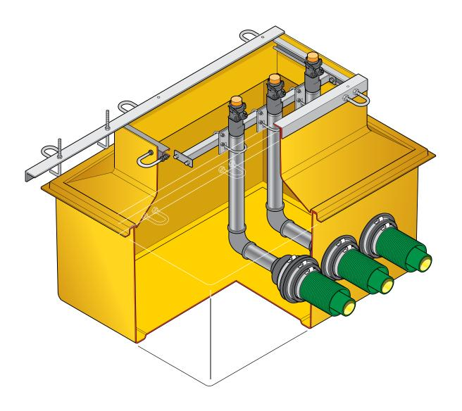
1100mm x 800mm GRP solid base sump and corbel to fit GobalStar 6 Hose dispenser. Side rail version.
