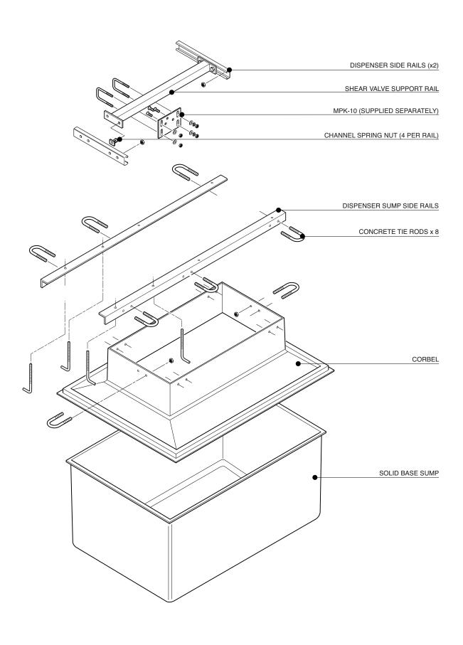
1100mm  $\times$  800mm GRP solid base sump and corbel to fit GobalStar 6 Hose dispenser. Side rail version.
