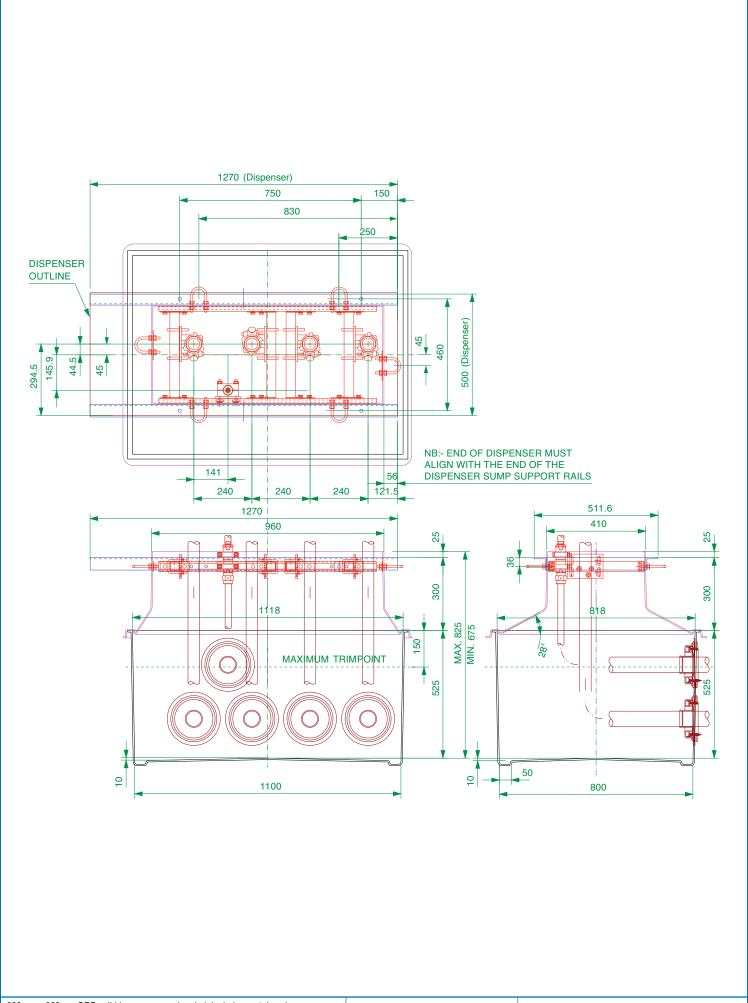
862mm x 862mm GRP solid base sump and corbel. Includes metal work.
