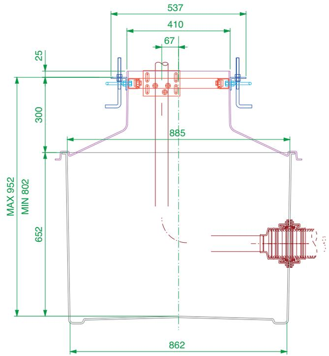
862mm x 862mm GRP solid base sump and corbel to fit Wayne Helix 2000 IEC, 2 diesel line model. Includes dispenser support rails, shear valve rails and all fixings.
