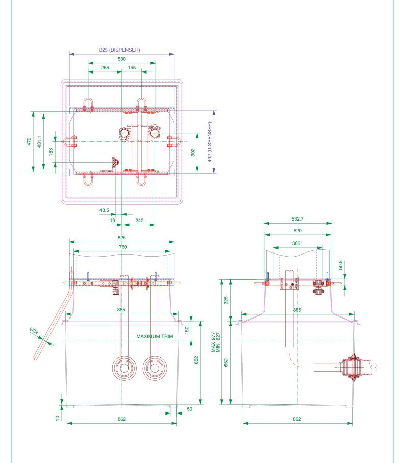
$862 mm \times 862 mm$  GRP solid base sump and corbel to fit Wayne HELIX dispenser model. Includes dispenser support rails, 2 shear valve rails and all fixings.
