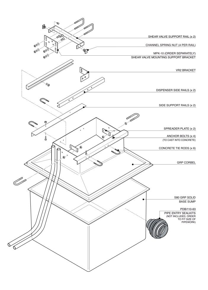
$862 mm \times 862 mm$  GRP solid base sump and corbel to fit Wayne HELIX dispenser model. Includes dispenser support rails, 2 shear valve rails and all fixings.
