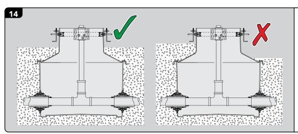
Backfill around the sump equally in levels to prevent uneven load against the sump wall.
