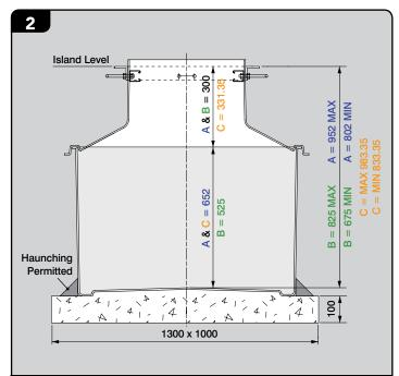
NB:- Sump should be embedded into the support base when installed.
