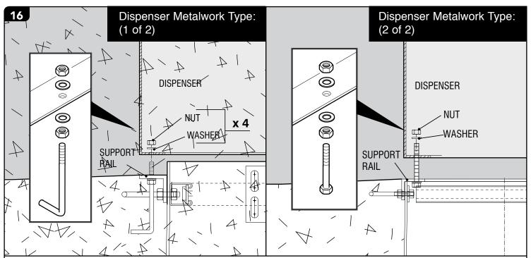
Remove upper nut & washer on the 4 anchor bolts. Install & connect the dispenser to the sump dispenser support rails & anchor bolt. Fit & tighten nut & washer.
