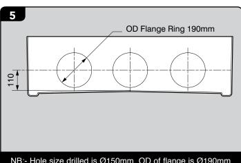
NB:- Hole size drilled is Ø150mm. OD of flange is Ø190mm
