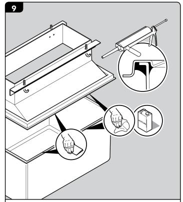
Abrade internal groove of corbel and top edge of the sump (inside & outside) with sandpaper. Degrease with acetone.
