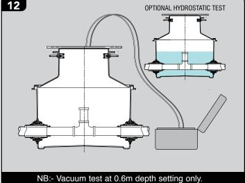
Optional vacuum water or hydrostatic test. Ensure pipework is capped off below the upward riser. Tighten clips on pipe entry sealkits against the pipe. Tighten nuts on upper support frame metalwork.
