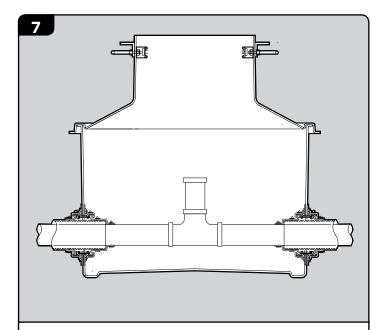
Run pipework through side wall and connect to upward riser. Cap off pipework to allow vacuum testing in stage 12.
