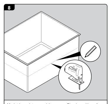
Mark trim point around the sump. Check position of pipe entry sealkits before trimming with a jig saw. Refer to stages 4 and 5 for pipework positions with and without trimming.
