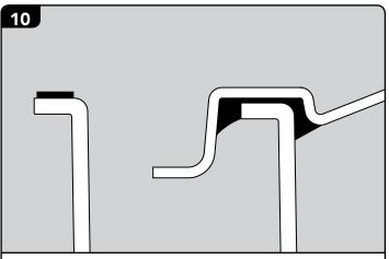
this has been removed during trimming, apply sealant the sump and push down firmly.
