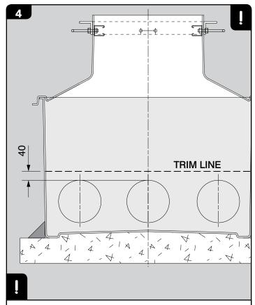
Before trimming the sump, ensure that all pipe seal kits are fitted and the position of the highest pipe seal kit flanges is at least 40 mm below the trim line.
