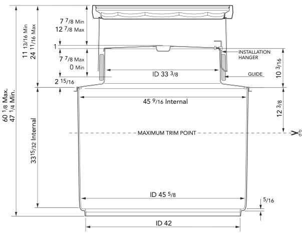
$45^\circ$  diameter sump to fit  $42^\circ$  tank collar ring with corbel, internal lid, adjustable skirt and round  $36^\circ$  flat sealed cover.
