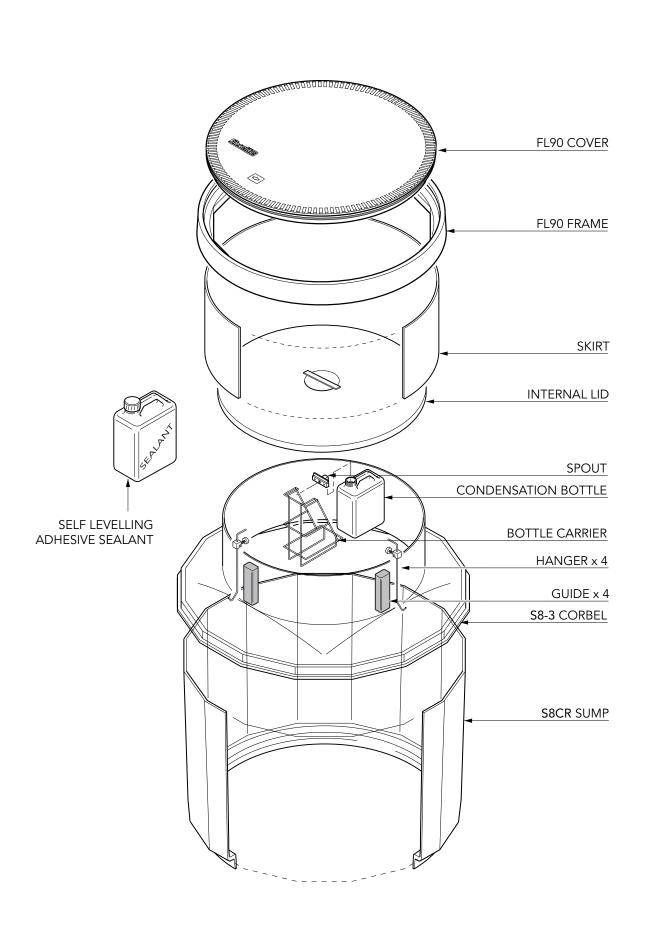
$45^{\circ}$  diameter sump to fit  $42^{\circ}$  tank collar ring with corbel, internal lid, adjustable skirt and round  $36^{\circ}$  flat sealed cover.
