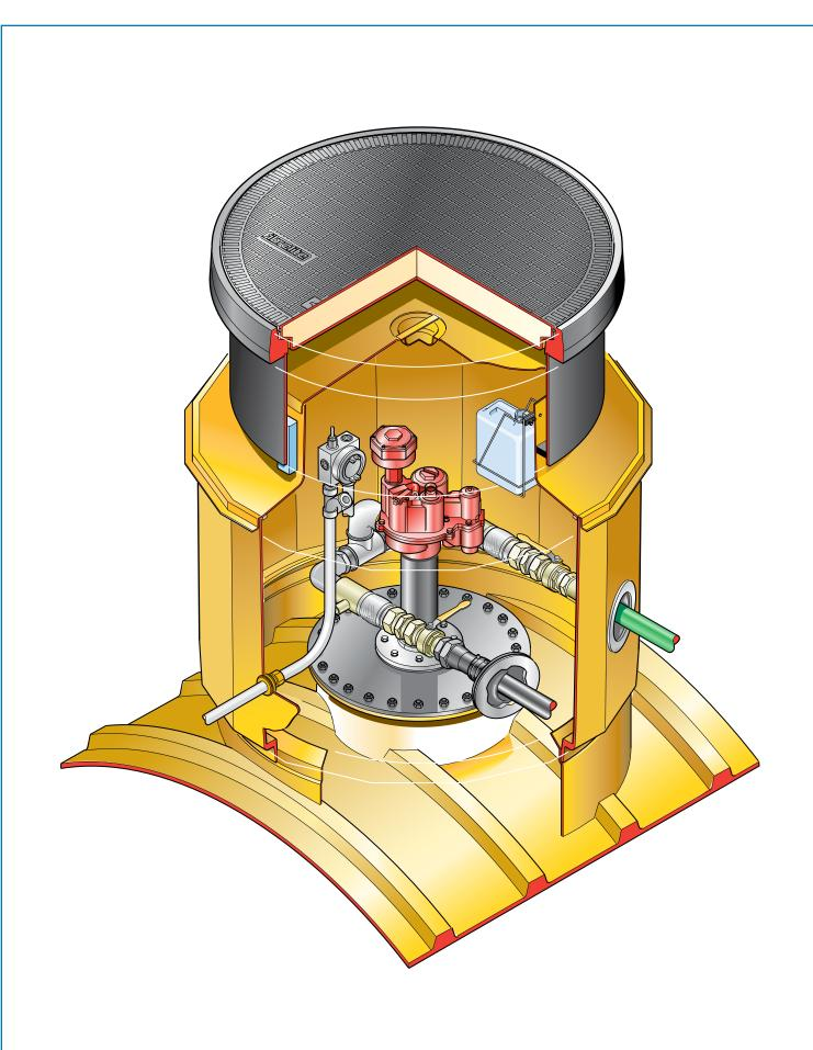
$45^{\circ}$  diameter sump to fit  $42^{\circ}$  tank collar ring with corbel, internal lid, adjustable skirt and round  $36^{\circ}$  flat sealed cover.
