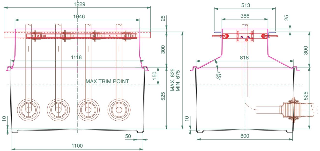
1100mm x 800mm GRP solid base sump and corbel to fit Wayne Vista 390 and 399 models. Includes metal work.
