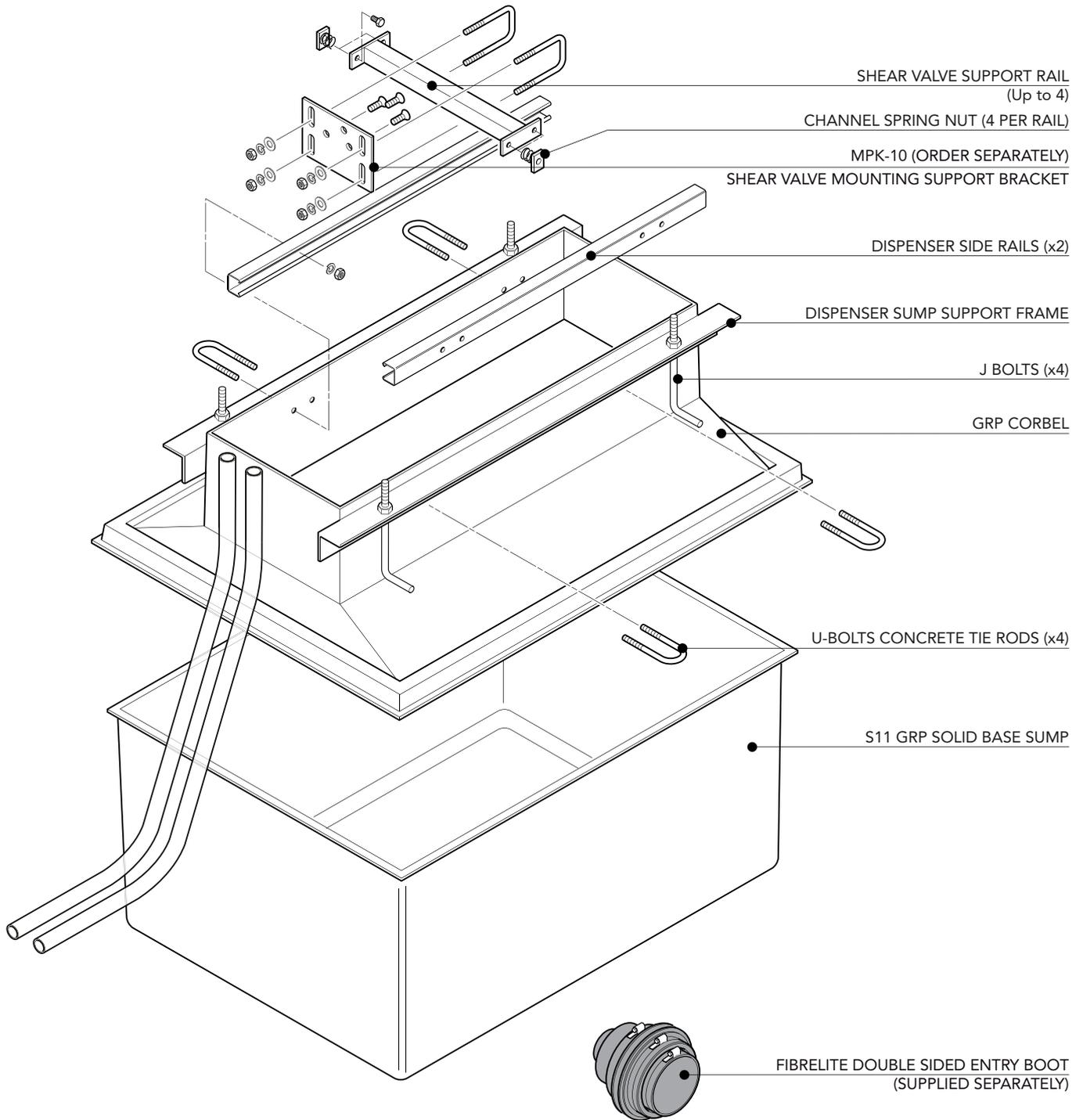
1100mm x 800mm GRP solid base sump and corbel to fit Wayne Vista 390 and 399 models. Includes metal work.
