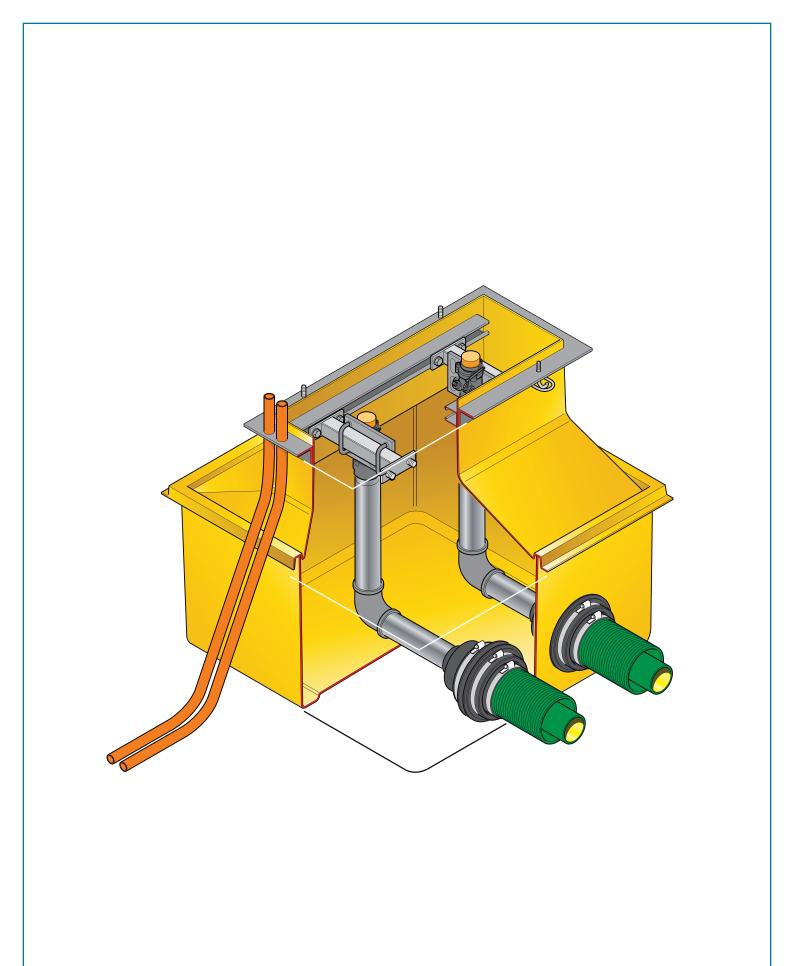
780mm x 780mm GRP solid base sump and corbel to fit Wayne Vista dispenser models with a narrow 35" body. Designed to fit between double canopy columns. Includes 2 dispenser support rails, 4 J bolts, 2 shear valve rails and 4 U bolts.
