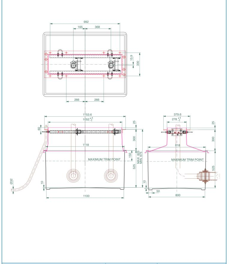
1100mm x 800mm GRP solid base sump and corbel to fit Wayne Vista wide body (48") models. Metalwork included.
