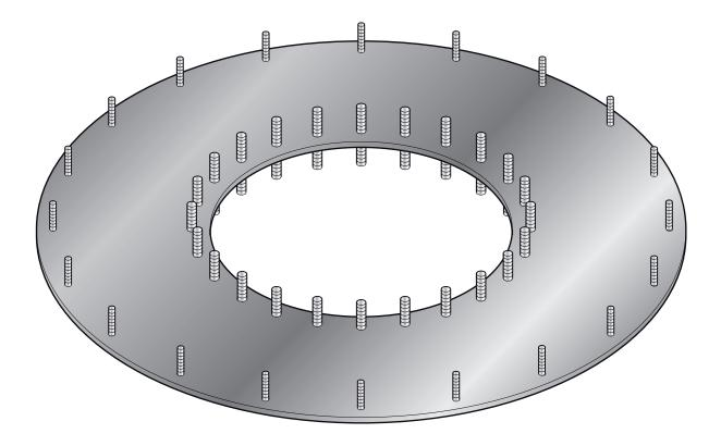
Steel adaptor plate with welded studs to connect the S14 chamber to a round tank manway lid. Various sizes available.
