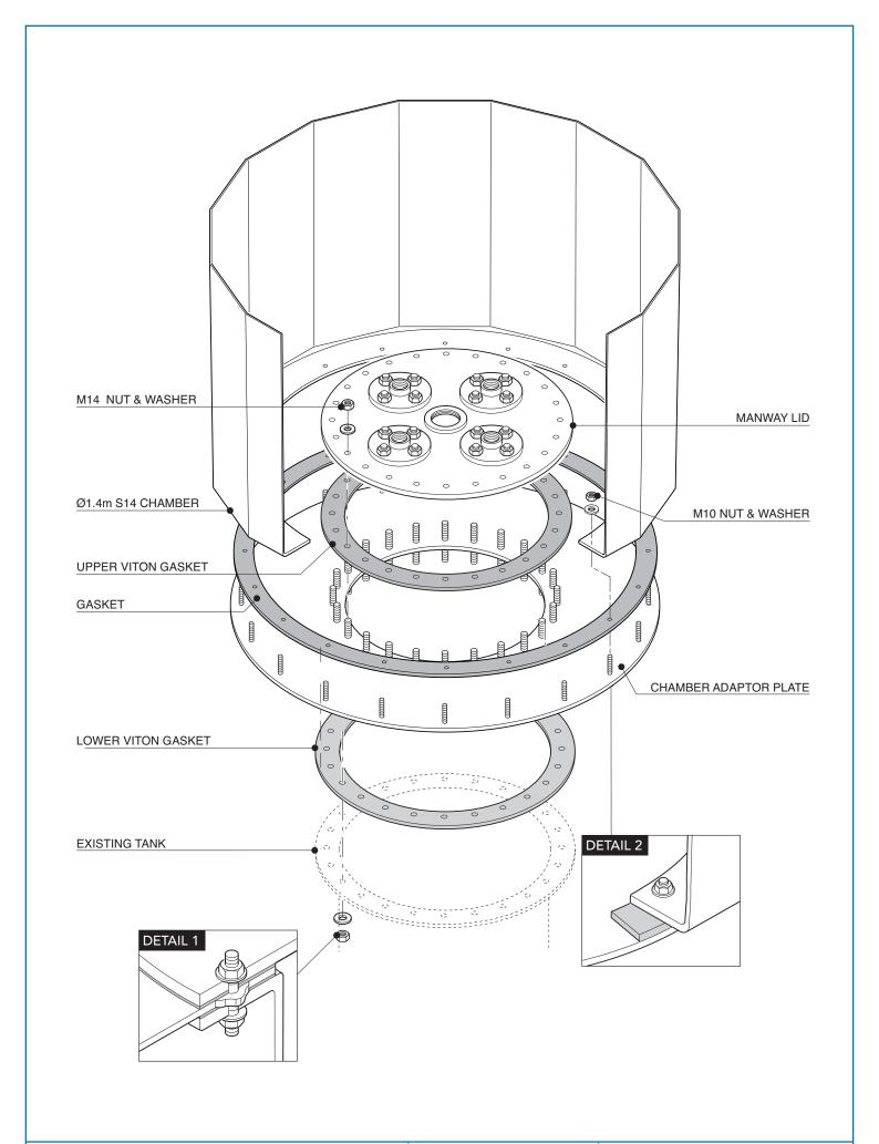
Steel adaptor plate with welded studs to connect the S14 chamber to a round tank manway lid. Various sizes available.
