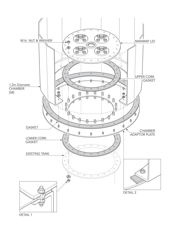
Steel adaptor plate with welded studs to connect the S8 chamber to a round tank manway lid. Various sizes available.
