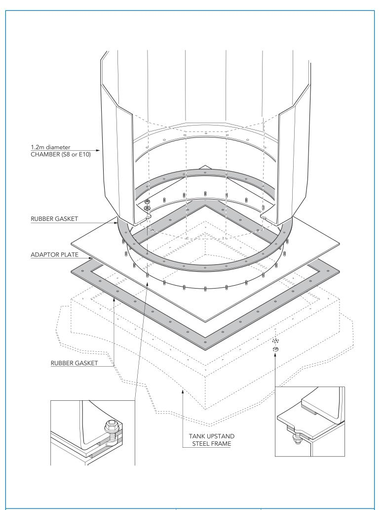
DIN bolt pattern adaptor plate to fit a round 1.2m dia. S8 chamber to a 1m2 upstand.
