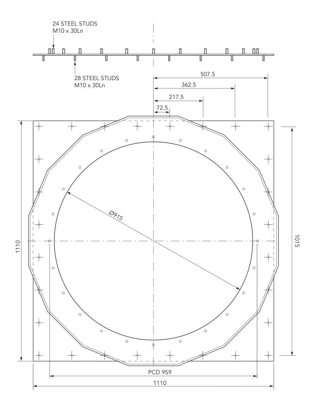
DIN bolt pattern adaptor plate to fit a round 1.2m dia. S8 chamber to a 1m2 upstand.
