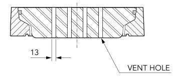
300mm diameter vented flat cover with composite frame. Temperature and chemical resistant. Designed for steam applications.
