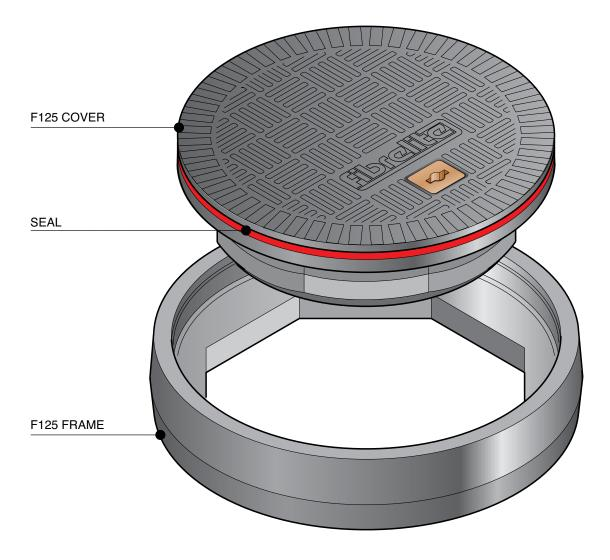
300mm diameter watertight flat sealed cover with composite frame. Temperature and chemical resistant. Designed for steam applications.
