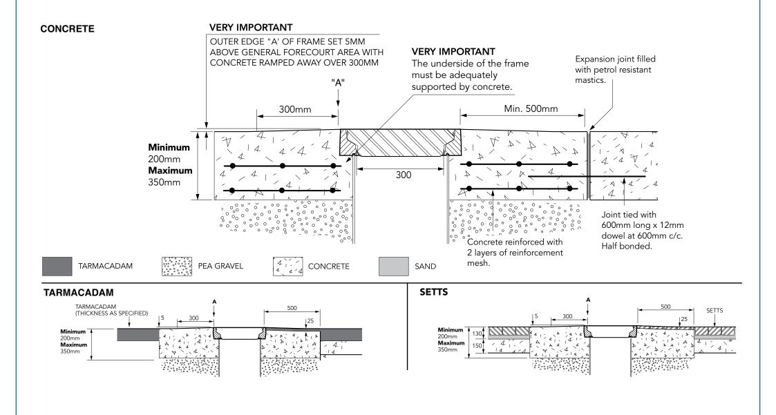
300mm diameter watertight flat sealed cover with composite frame. Temperature and chemical resistant. Designed for steam applications.
