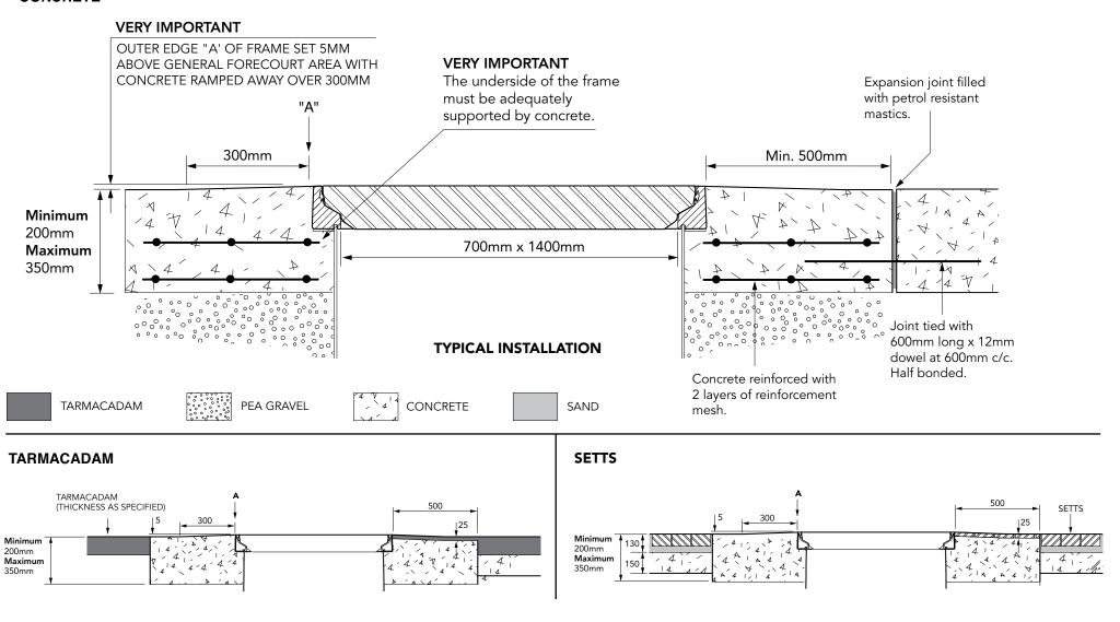
1400mm x 700mm flat, vented composite cover with aluminium frame. Temperature and chemical resistant. Designed for steam applications.
