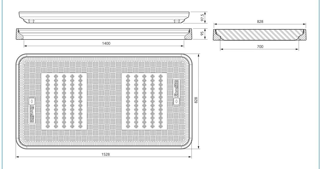
1400mm x 700mm flat, vented composite cover with aluminium frame. Temperature and chemical resistant. Designed for steam applications.
