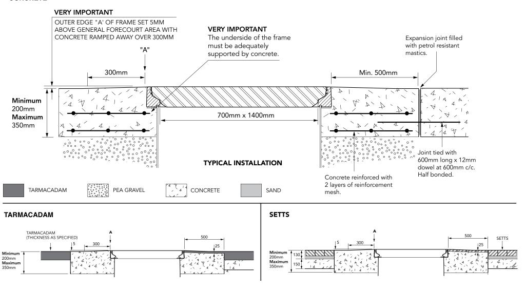
1400mm x 700mm flat sealed composite cover with aluminium frame. Temperature and chemical resistant. Designed for steam applications.
