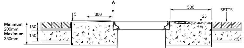
457mm x 457mm square vented flat composite cover with composite frame. Temperature & chemical resistant. Designed for steam applications.
