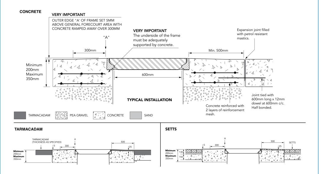
600mm x 600mm flat sealed composite cover with an aluminium frame. Temperature & chemical resistant. Designed for steam applications.
