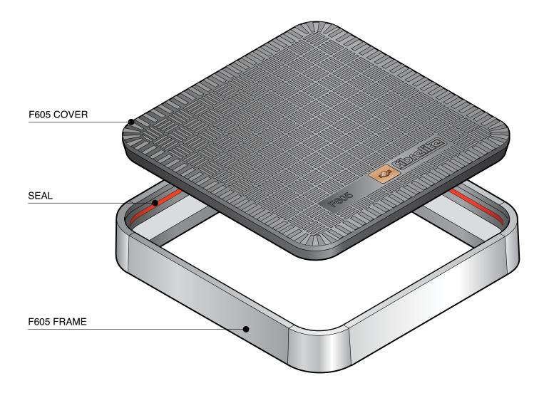
600mm x 600mm flat sealed composite cover with an aluminium frame. Temperature & chemical resistant. Designed for steam applications.
