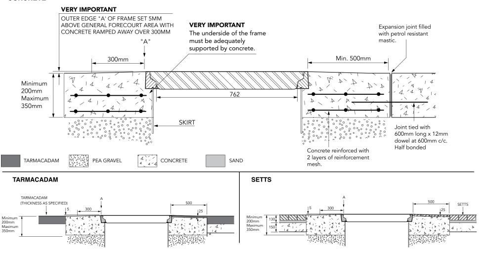
760mm diameter flat sealed composite cover and composite frame. Temperature and chemical resistant. Designed for steam applications.
