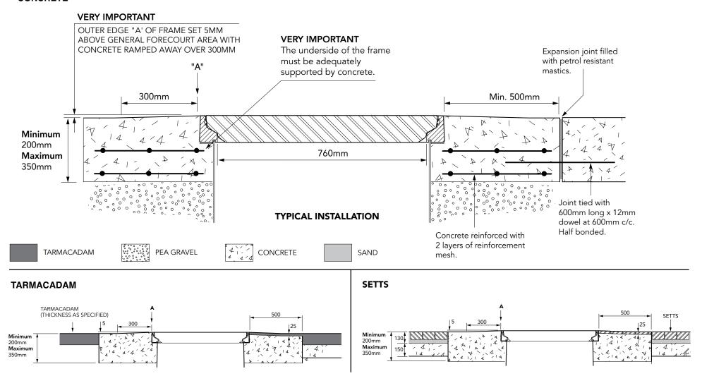
760mm square watertight flat sealed cover with an aluminium frame. Temperature & chemical resistant. Designed for steam applications.
