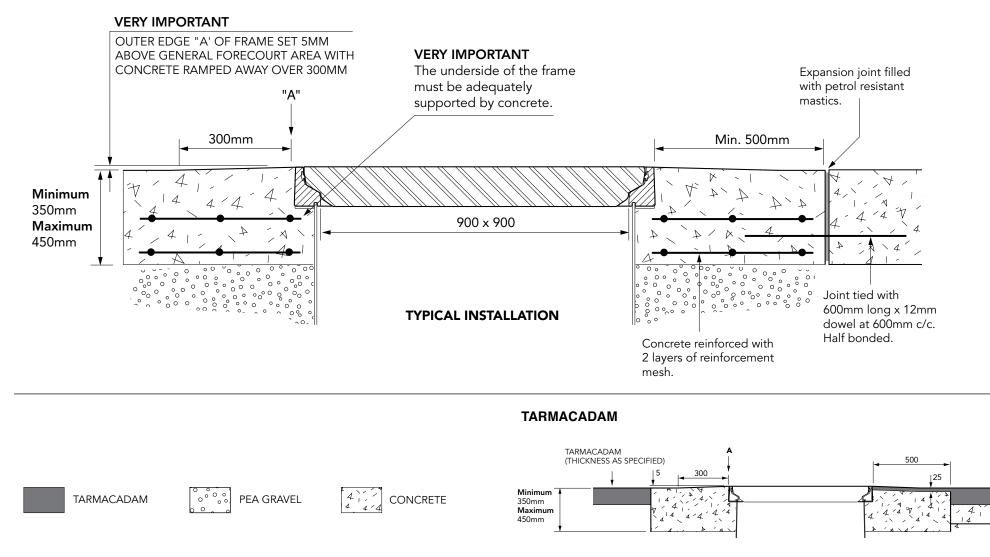
900 mm square flat sealed composite cover with an aluminum frame. Temperature & chemical resistant. Designed for steam applications.
