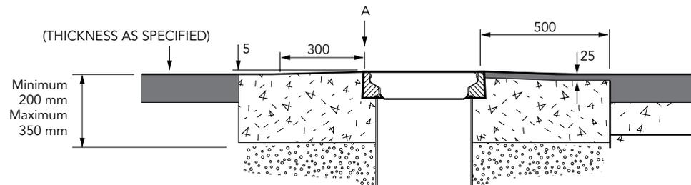
300mm diameter flat sealed composite cover with a Grounding Point ID and a composite frame.
