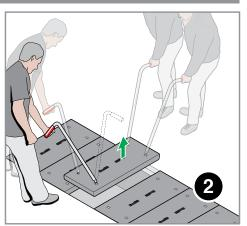
Simultaneously pull the cover upwards.
