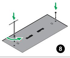
Using the T-bar, replace the 2 No. restraining bolts.
