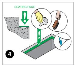
Clear and clean the frame or rebate, particularly the seating face. Inspect for damage.
