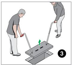
Simultaneously pull the cover upwards.
