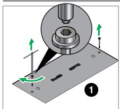
Using the T-bar Allen Key, remove the 2 No. restraining bolts.
