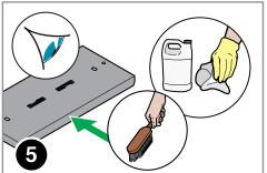
Clean the cover using only warm water and standard cleaning detergents. Inspect for damage. Frequency depends on use and the working environment but it is recommended that cleaning and inspection are carried out at least once every 6 months. It is recommended that spillages are clean up immediately.
