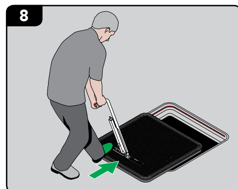
Align correctly with frame. Push cover into position using your foot.
