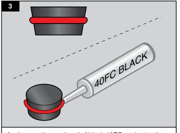
Apply a continuous bead of black 40FC sealant to the outside diameter of the rubber plug.
