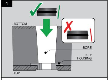
Insert the rubber plug, narrow end first into the key housing bore until it engages on the taper.
