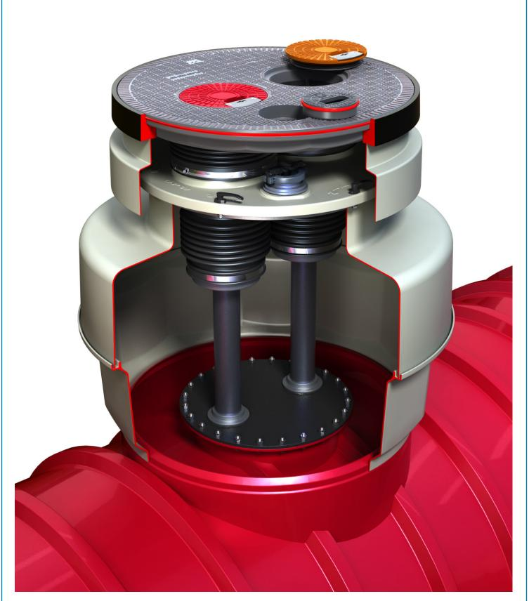
48" medium bury collar mount sump base, tophat, watertight platform for (2) 5-gallon spill buckets, skirt, cover frame, 40" diameter multiport cover and port covers.
