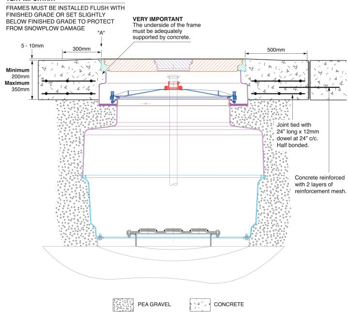
1.2m medium bury reverse flange sump base to fit tank upstand,tophat, watertight platform, skirt, cover frame and 1020mm diameter centre port cover and port cover. For Elutron Mexico.
