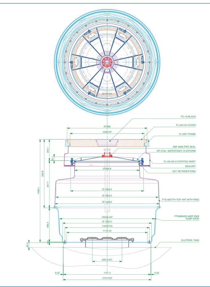
1.2m medium bury reverse flange sump base to fit tank upstand,tophat, watertight platform, skirt, cover frame and 1020mm diameter centre port cover and port cover. For Elutron Mexico.
