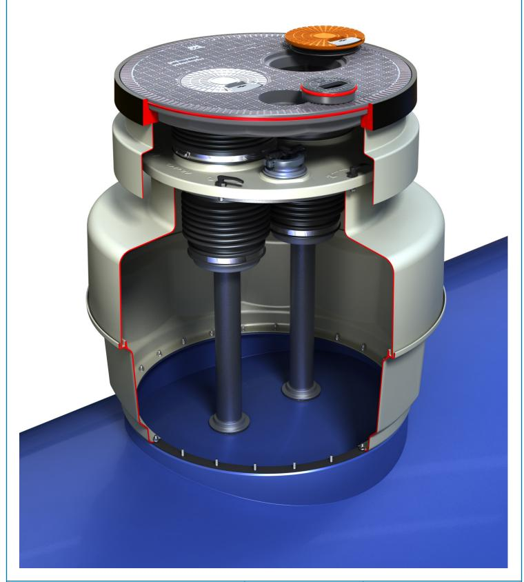
1.2m medium bury reverse flange sump base to fit tank upstand, tophat, watertight platform for (2) 5-gallon spill buckets, skirt, cover frame, 1020mm diameter multiport cover and port covers. For Elutron Mexico.
