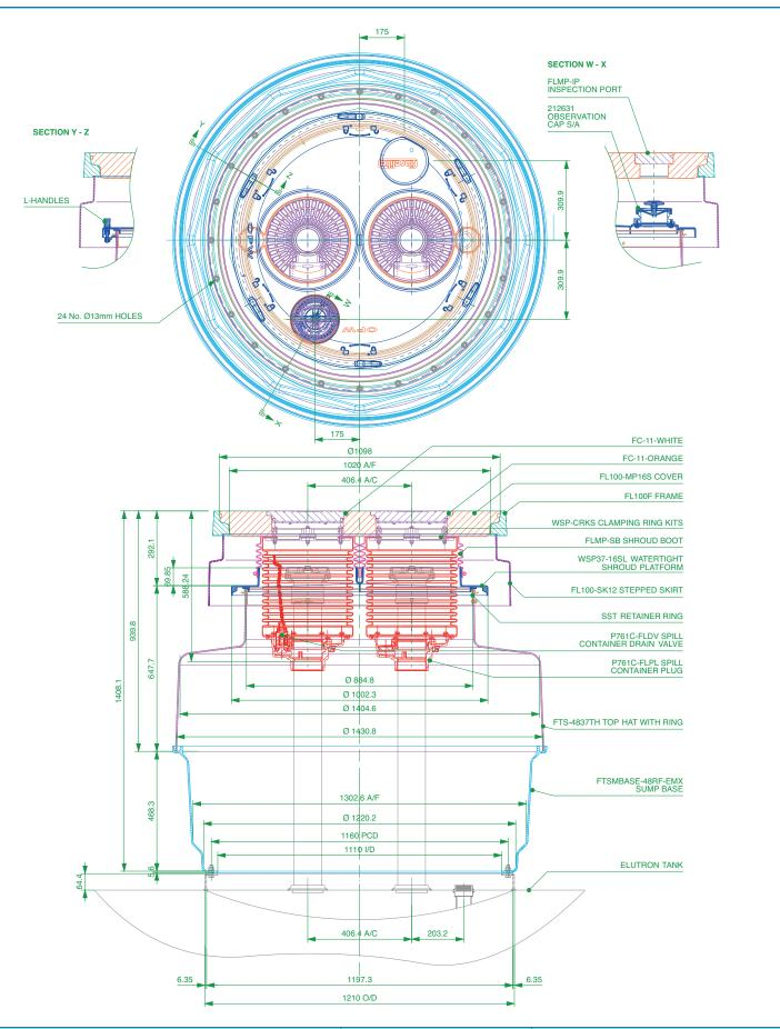
1.2m medium bury reverse flange sump base to fit tank upstand, tophat, watertight platform for (2) 5-gallon spill buckets, skirt, cover frame, 1020mm diameter multiport cover and port covers. For Elutron Mexico.
