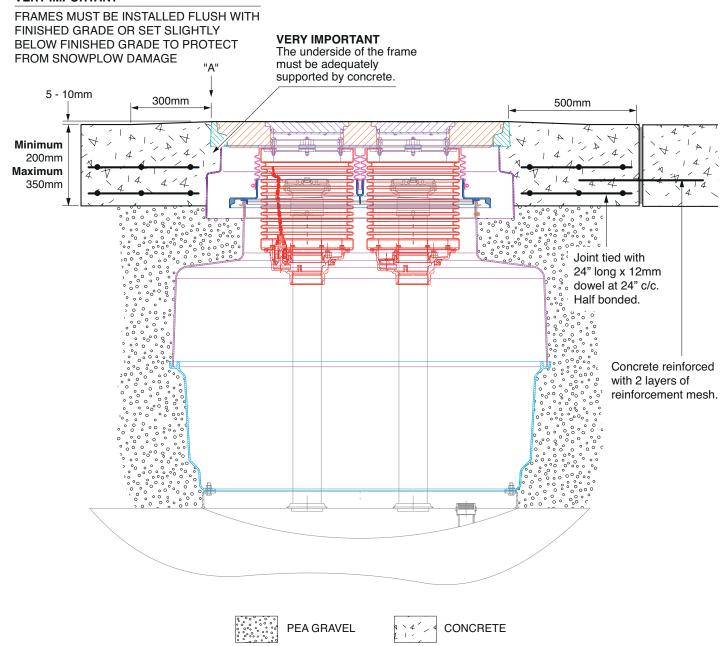
1.2m medium bury reverse flange sump base to fit tank upstand, tophat, watertight platform for (2) 5-gallon spill buckets, skirt, cover frame, 1020mm diameter multiport cover and port covers. For Elutron Mexico.
