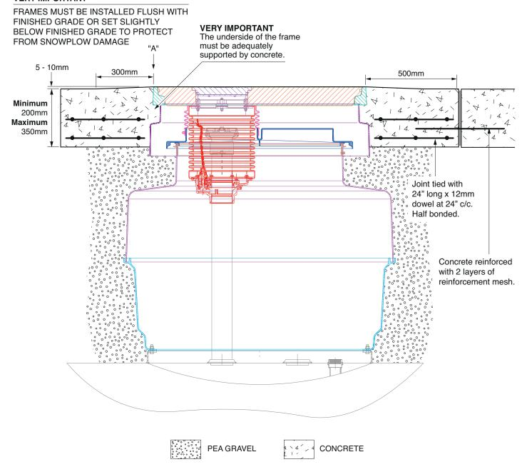
1.2m medium bury reverse flange sump base to fit tank upstand, watertight platform for (1) 5-gallon spill bucket, skirt, cover frame, 1020mm diameter offset port cover and port cover. For Elutron Mexico.
