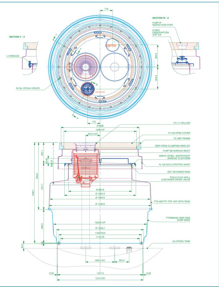
1.2m medium bury reverse flange sump base to fit tank upstand, watertight platform for (1) 5-gallon spill bucket, skirt, cover frame, 1020mm diameter offset port cover and port cover. For Elutron Mexico.
