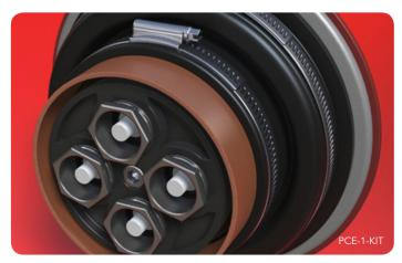
Fibrelite's range of pipe and cable entry kits offer a unique design allowing a single hole installation. No additional screw holes need to be drilled. This provides the installer with a quick and easy installation and minimises potential leak paths through the sump wall. The pipe sleeves are made from a fuel resistant nitrile grade or Viton rubber and the bellowed design facilitates movement with changing ground conditions.
