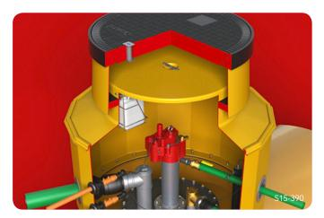
Manufactured using the latest in FRP technology, Fibrelite offers a range of sumps for any type of tank connection. They are all height adjustable allowing easy installation and eliminate any load transfer from the cover to the tank. Available round, square or rectangular, all sumps are supplied in multiple pieces creating the maximum space for installers to work.
