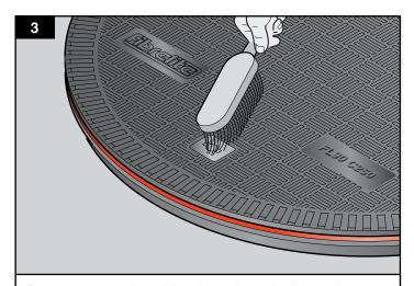
Do not remove the rubber bung from the base of the cover key housing. Remove debris from the key housing with suitable tools.
