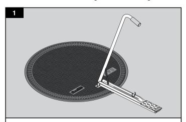
The purpose designed lifting aid (FL7A) must be used at all times to remove and replace the Fibrelite cover. Failure to use the specifically designed lifting aid may result in damage to the cover and injury.
