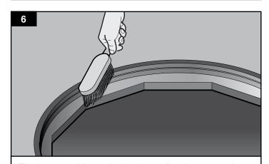
The frame and in particular the sealing faces must be kept free from debris as this may damage the seal and compromise the covers water tight effectiveness. It is recommended that the frame be cleaned with a brush during removal and replacement.
