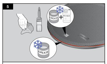
It is recommended that the key housing be filled with grease and antifreeze and the seal be coated in grease in climates that drop below freezing (0°C - 32°F). If grease is applied to the cover seal it must be a non-petroleum based grease, preferably silicone.
