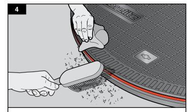
Ensure that the seal and sealing faces of the cover are clean and free from debris as this may damage the seal and compromise the covers water tight effectiveness. It is recommended that a soft bristle brush or clean rag be used to clean the cover.
