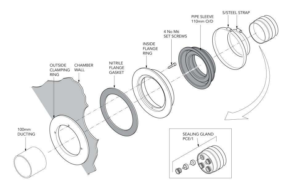
110mm dia. pipe entry seal kit (PSB/110),with sealtight compression gland. Sealing gland fits 4 cables (9-20mm) or 12 cables (4-8mm). Internal sealing gland can be purchased separately. (PCE/1)
