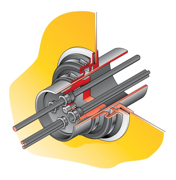
110mm dia. pipe entry seal kit (PSB/110), with sealtight compression gland. Sealing gland fits 4 cables (9-20mm) or 12 cables (4-8mm). Internal sealing gland can be purchased separately. (PCE/1)
